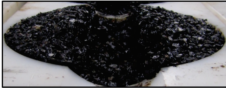
Figure 2.7. Typical tested APA specimen.
