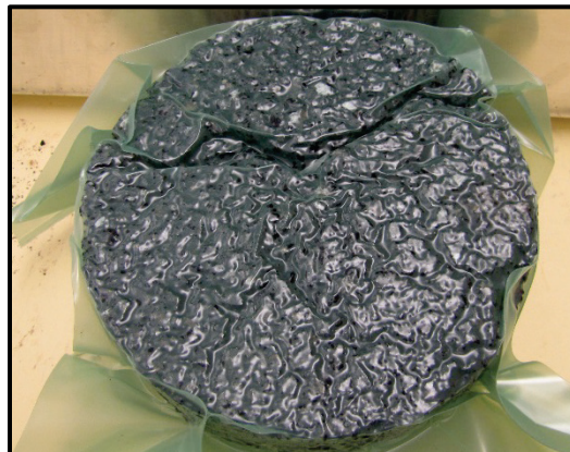
Figure 2.5. Typical cold mix specimen deformed by CoreLok bag.
